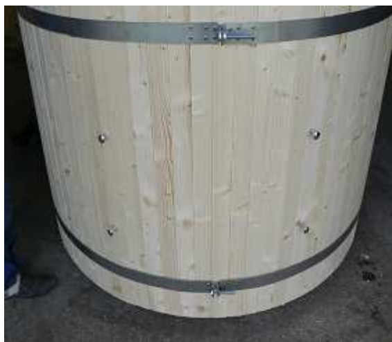
Photo 13. Fastening bolts of the furnace
